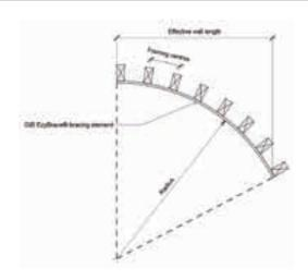
the application method in this bulletin. The curving must not weaken or crack the gypsum core. The projection of a curved GIB EzyBrace® bracing element should be used as the effective wall length, as illustrated below.
