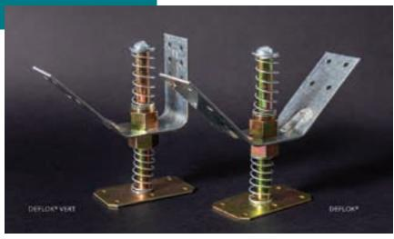
The DEFLOK® solution is an elegant, tested and sealed unit that accounts for a full + or – 35mm of vertical movement. It has been physically tested, to have 241 KGF of capacity through the full range of vertical movement.
